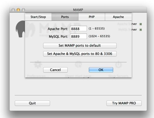
Server programs, when addressed via the network, need to be assigned to a certain network port. This way, multiple server programs may run on one server machine. Every service has a default port: The Apache web server typically uses port 80, the MySQL database server utilises port 3306.
